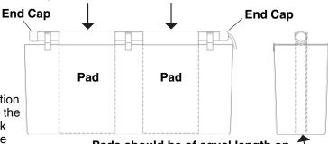
Pads should be of equal length on each side of the heater bar.
